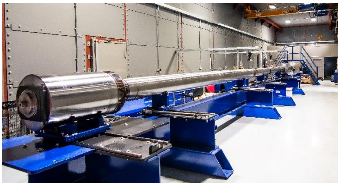
Fig. 3 - The Two-stage Light Gas Gun used to Accelerate Projectiles Up to 6.5 km to Achieve Projectile Fusion (©First Light Fusion Limited, 2021)
