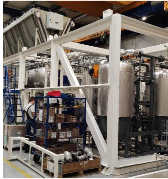
Picture 4: Hydrogen generator PEM technology at the assembly line in Rockfin S.A.
