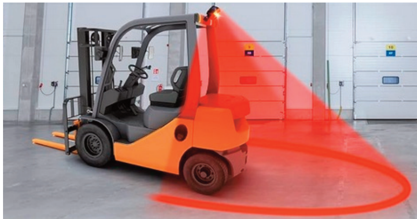
Example of marking a hazardous zone in the vicinity of a forklift truck.
