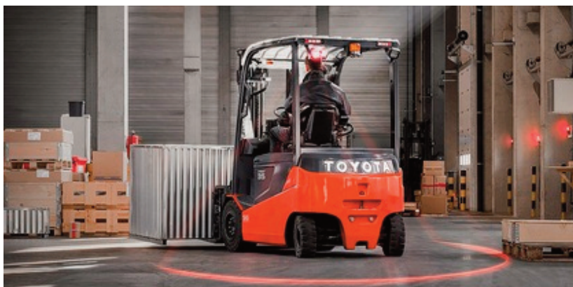
Example of a forklift truck with a designated danger zone
