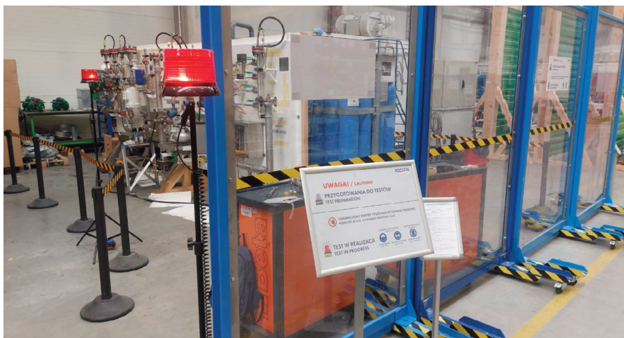
An example of a dedicated tests zone with protection borders
