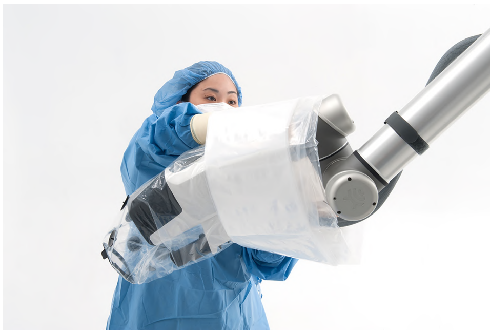
Figure 33 Drape over end effector
