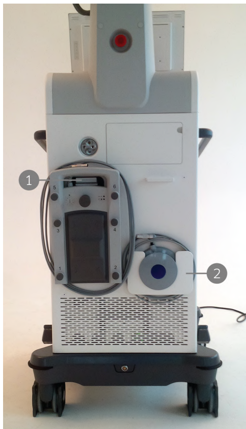
Figure 16 Pedals stowed in mobile base
