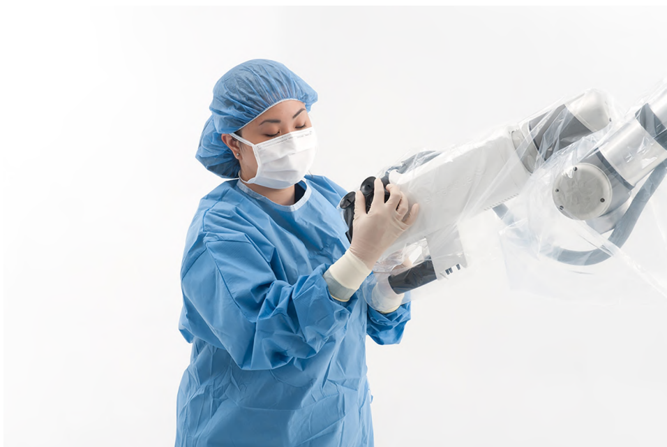
Figure 34 Pressing the marker posts onto the end effector
