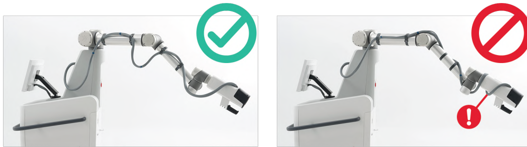
Figure 11 Correct and incorrect cable positions. The red callout indicates incorrect cable positioning wrapped around the end effector.
