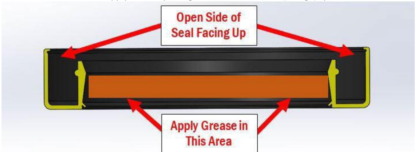
Figure 35: Seal Orientation and Grease Location
