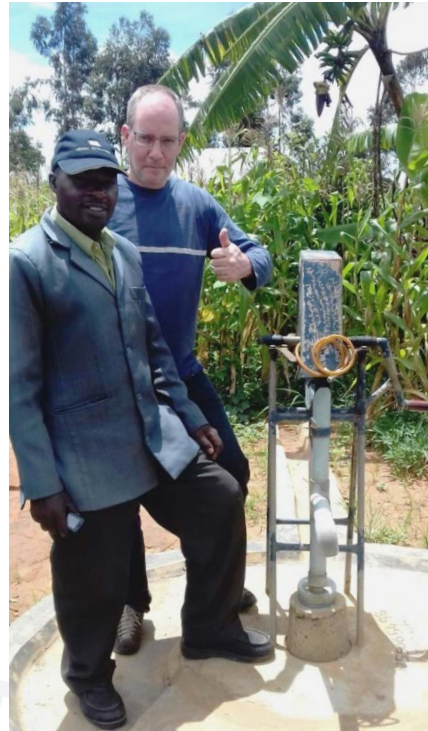
Mr. Hari and Matthias Saladin at a rope pump (Tanzania) constructed by Hari and his team
