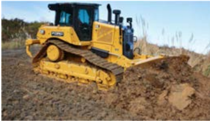
Figure 4: Example of types of bulldozers that would be used for site clearing works
