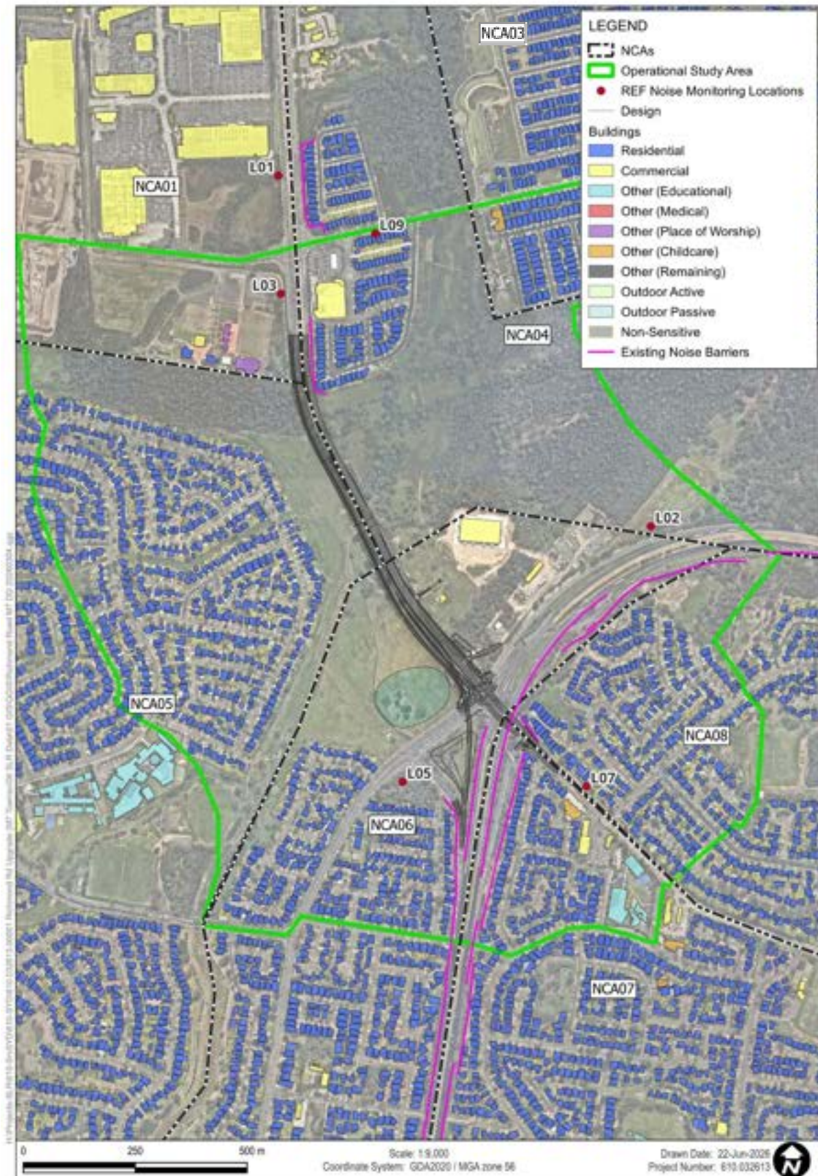
Figure 2 Receiver and Noise monitoring Locations
