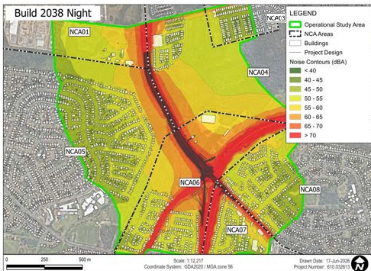
Figure 4 Predicted Operational Noise Levels with Project (Night-time Scenario 2038)
