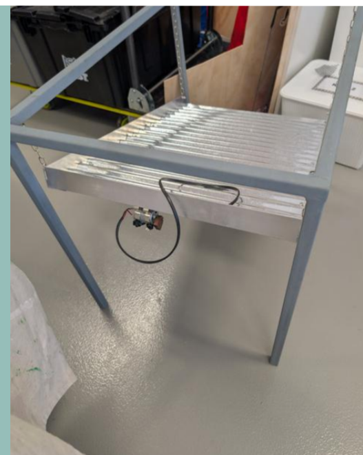
Images 21: Year 7/8 students have been hands-on with engineering challenges. They constructed jig tables to model how gold is separated from ore, studying the physics of movement and density, and linking this to how gold moves naturally in rivers and streams. They also designed creative Rube Goldberg machines to demonstrate how simple machines can move objects, connecting this concept to the gold mining process.
