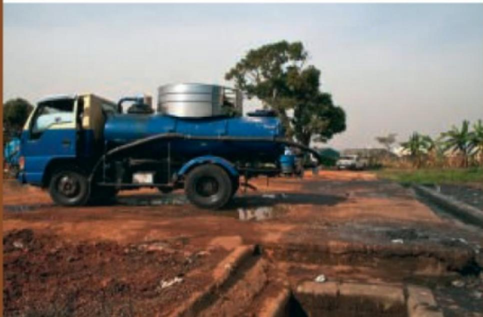
The practical extra structure on the top makes storage of the hose during transfers blindingly easy.
