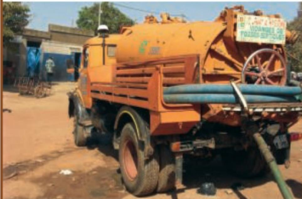
The Berliet vacuum truck stands out with its characteristic rear end closing wheel.
