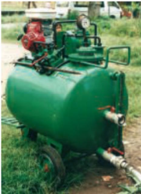
The vacuum tug used in Hải Phòng transfers the sludge from households that are difficult to access to a container in the streets.
