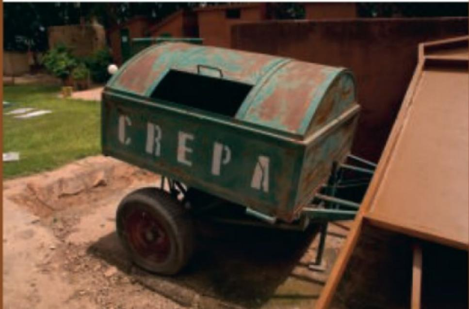
This hand cart transports sludge from latrines to the transfer station.
