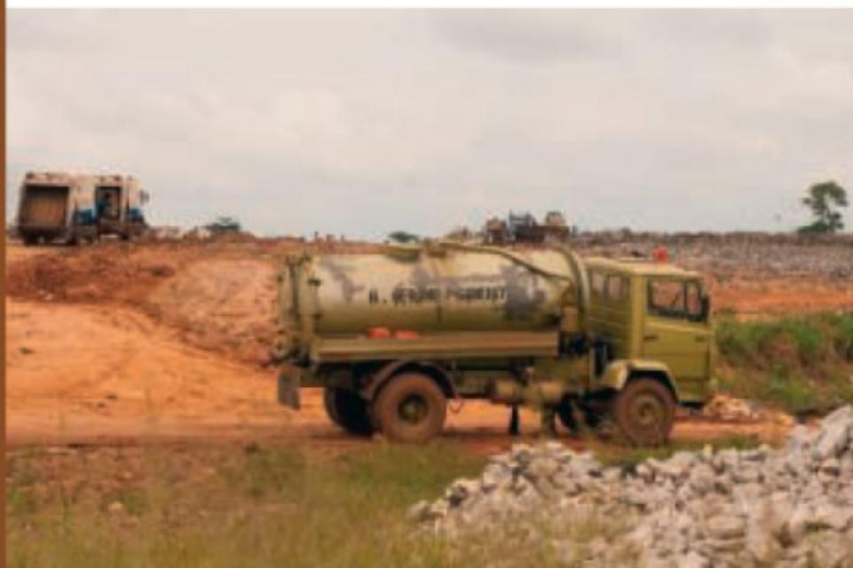
With its huge chassis clearance, the SINOTRUCK is well adapted to sludge disposal near landfills.
