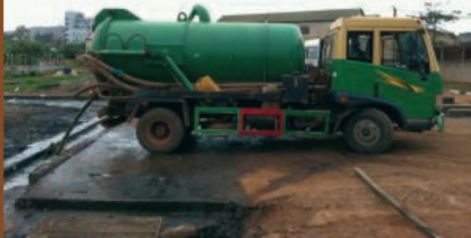
The vacuum pump can lift the sludge from tanks as deep as 6 m.
