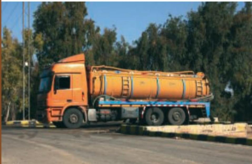
This large suction truck is well chosen when septic tanks are easily accessible from the road.
