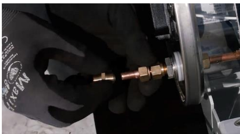
Figure33 - Manifold Connection via 10mm to 8mm reducer Compression Fitting
