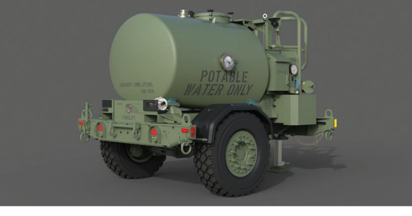
ND Defense's Bulk Potable Water System has a 530-U.S. gallon tank, which delivers:
