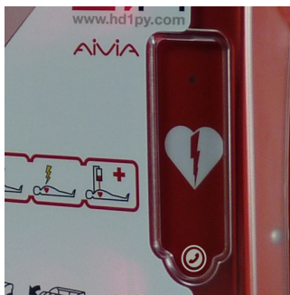
Call button to activate GSM hands free telephone module.
