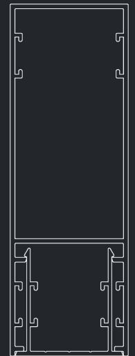
ASSEMBLED BATTEN 150MM X 50MM
