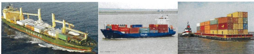
Figure 6 Sub-Panamax Multi-Purpose/Combo and Container Feeder Ships and Coastal Container Barge
