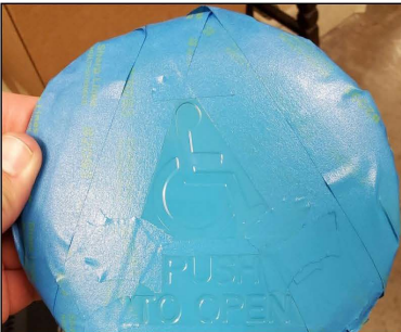
Let the paint dry for approx 24 hours. (seriously if you touch the paint or fiddle with it, it can ruin the surface finish and you will have to start the process over.)
