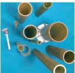
Filament wound tubes and shapes have exceptional interlaminar shear strength. Glass/epoxy resin ratios, winding tensions and pre-determined wind angles give directional strength as required for each application. Tubes weighing half as much and with equal strengths as similar size aluminum tubes may have 33% thinner walls. Glass/epoxy filament wound tubes can be machined to close tolerances.
