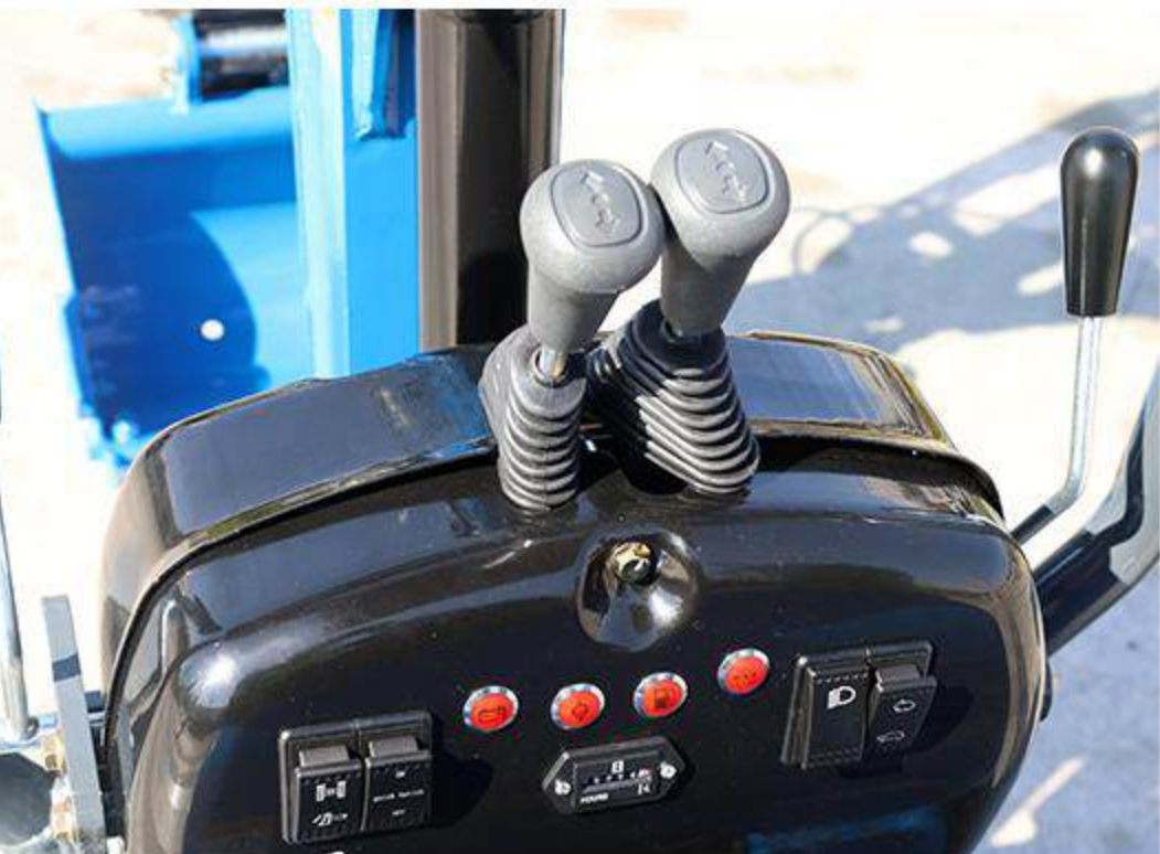
1 Front-mounted control lever The front-mounted operating lever ensures ample space for the feet and around the driver's seat.
