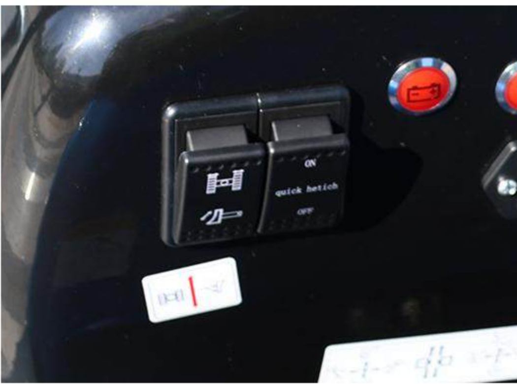
6 Multi-function button The crawler extension and dozer blade switching functions can be realized through simple button operation, as well as the quick change of attachments.
