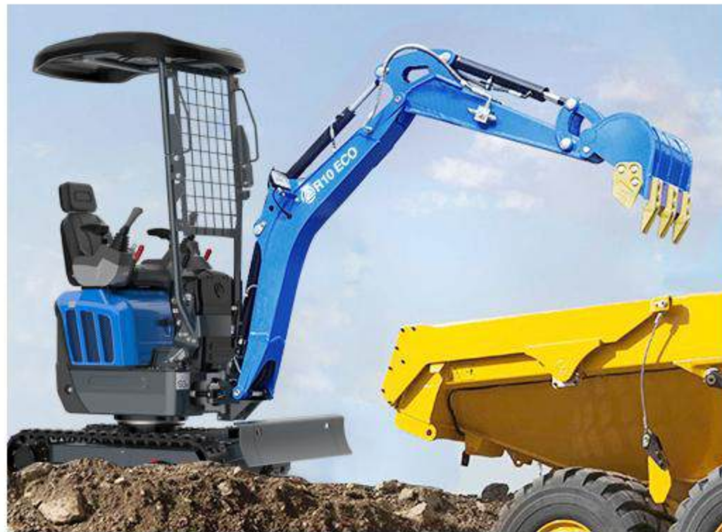
10 Rear boom cylinder You can scoop up large stones and concrete pieces with the bucket, load them onto a dump truck, or work with a mounted breaker without worrying about damaging the boom cylinder.
