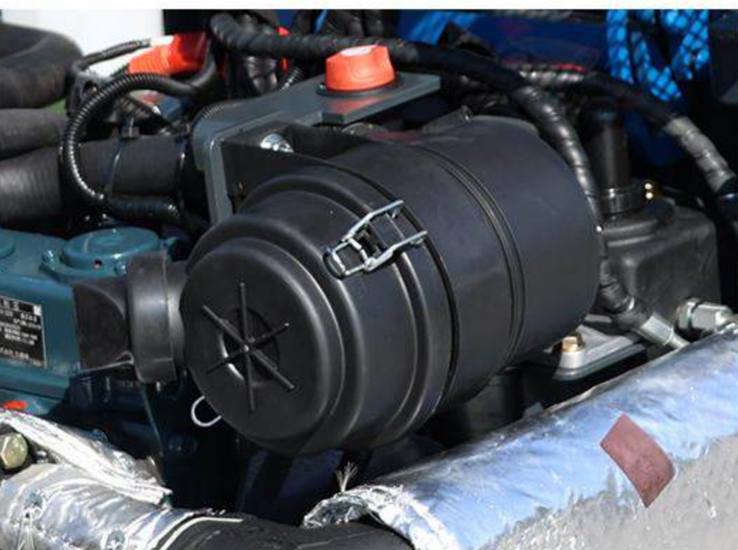
5 Air Filter Prevent dust and impurities from entering the engine's air intake system, thus extending the engine's service life
