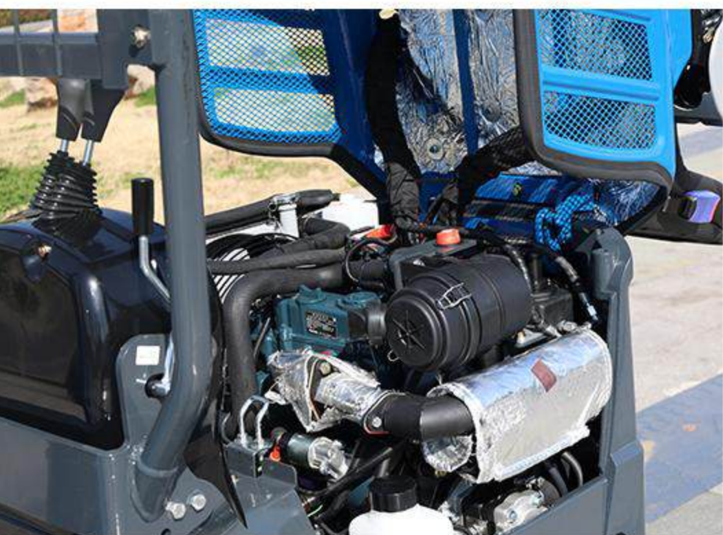
3 Fully openable bonnet The fully-opening bonnet opens wide to the rear, making it easy to carry out daily inspections and part replacements around the engine and fuel system.
