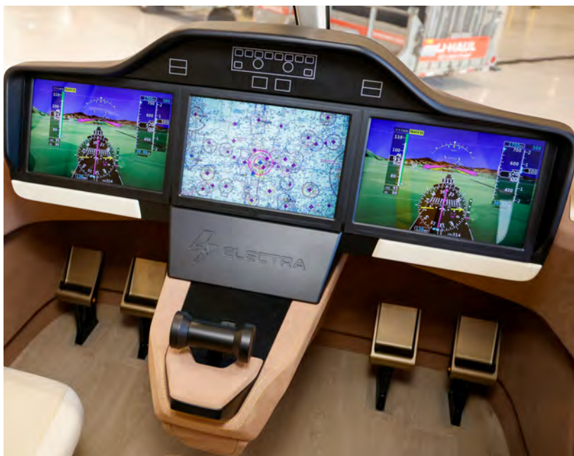
A mockup of the Electra EL9 shows that the commercial aircraft will have nine passenger seats, glass-panel avionics with synthetic vision, autothrottles, and side sticks for the computerized fly-by-wire control system. The avionics suite is meant to boost pilot situational awareness regardless of whether they're operating from busy airports or remote fields.
