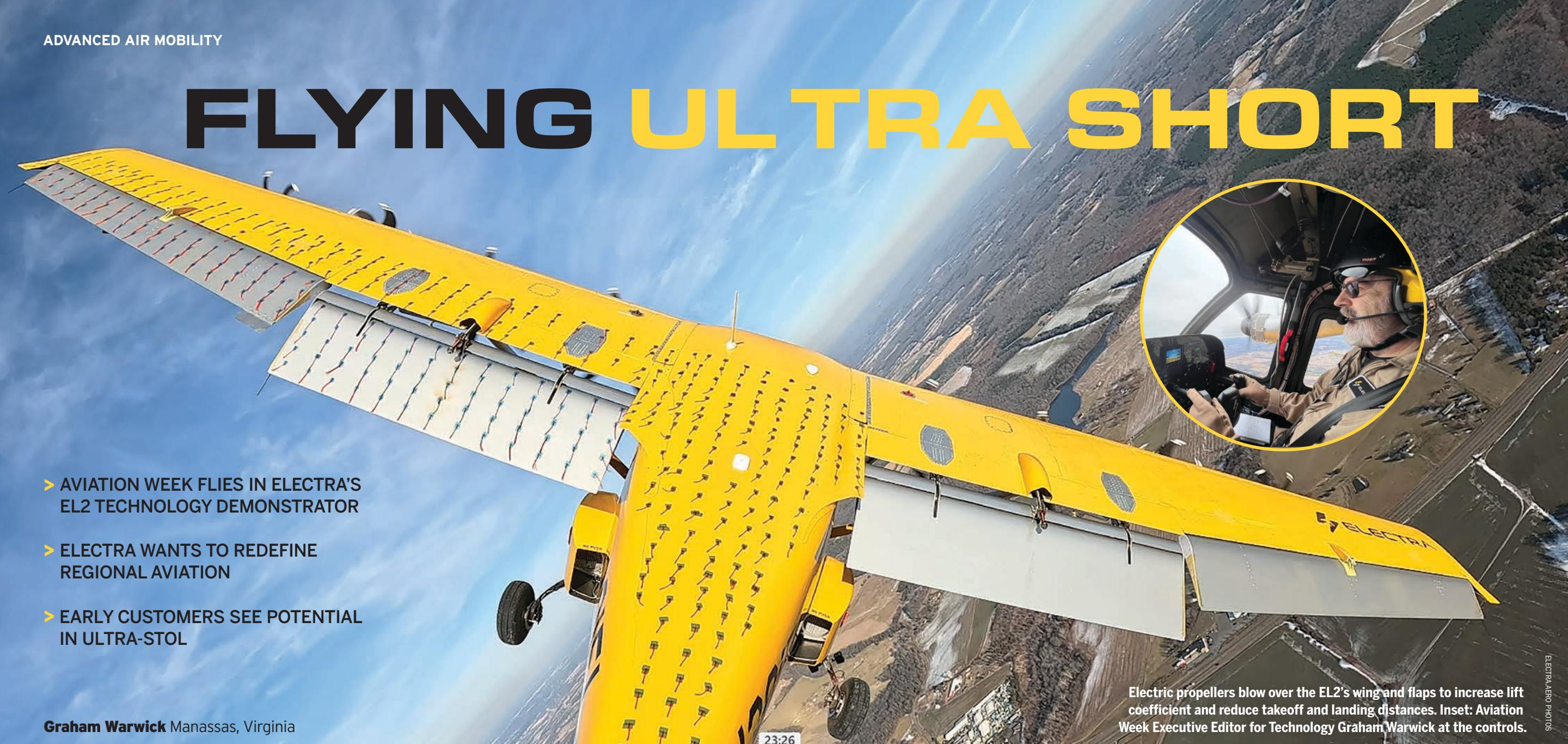
reduce drag and helps dampen the effects of turbulence. The EL2's donor 172 wingbox has a break at about two-thirds span and is tapered outboard, so the outer pairs of propellers are smaller to avoid overblowing the outboard sections. All eight propellers are powered by the same MAGiCAll motors. On the production EL9, all eight propellers will be identical.
