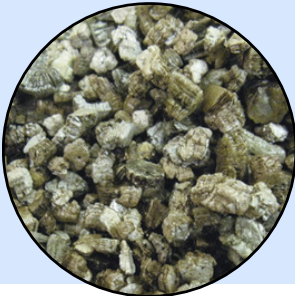
VERMICULITE / BLOWN INSULATION
