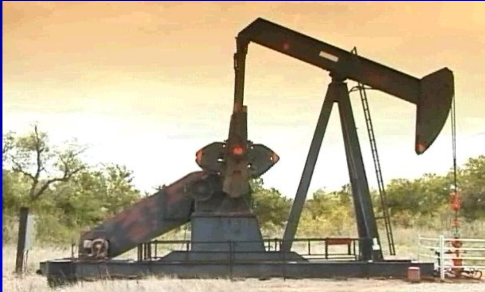
For safety purposes after stopping the unit set the brake and disconnect power.
