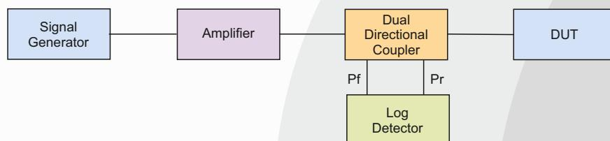
Recently directional coupler and log detector used to measure the forward and reflected power in a RF system. The block diagram is shown as above
