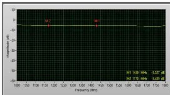
Graphs shows attenuation of pi attenuator. It shows -5.5dB attenuation over the entire frequency band from 1000MHz-1800MHz
