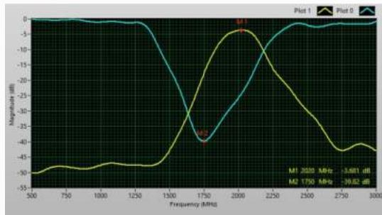
Graphs show transmission and reflection coefficient of filter. It can conclude that the transmitted power (S12) is -3dB and reflected power (S11) of filter is very less around -39.8dB.
