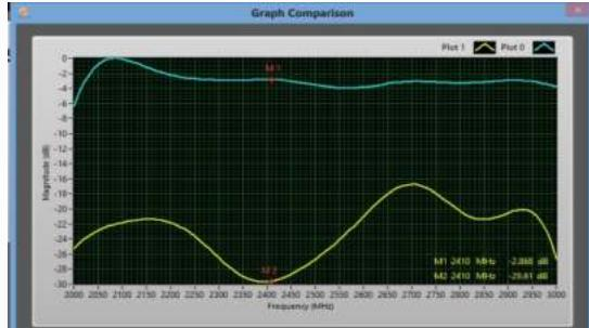
Graphs show both Insertion loss (S31) and Mutual coupling (S41) of hybrid coupler. The yellow graph shows isolation of coupler is -29.6dB and Blue graph shows insertion loss of coupler is -2.8dB at 2410MHz
