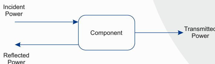
$$\text{Insertion Loss} = \frac{\text{Transmitted Power}}{\text{Incident Power}}$$
