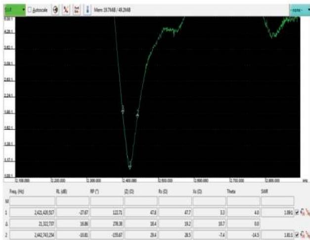
Graph shows the VSWR of patch antenna and its VSWR value is 1.09 which is nearly equal to ideal value 1.
