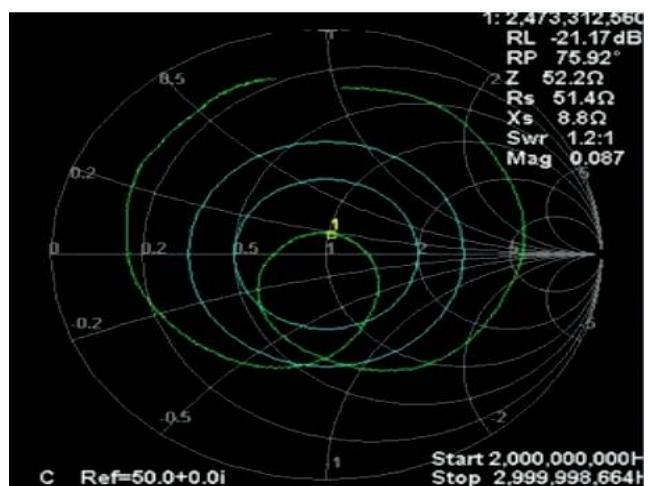
Graphs shows smith chart of antenna and its shows impedance of antenna is around 52 ohm
