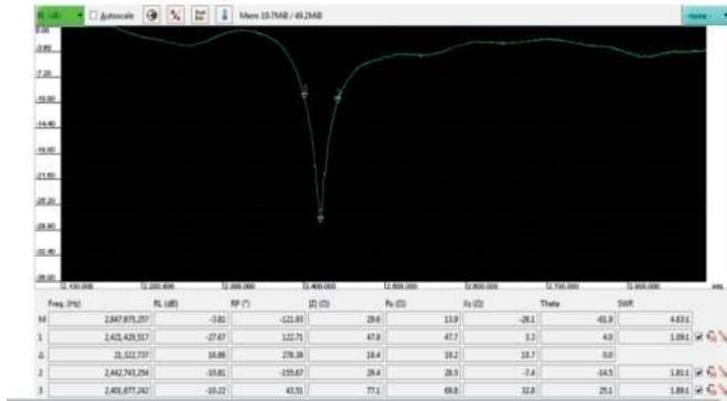
Graph shows return of patch antenna and its return loss value is -27.67dB at frequency 2421 MHz
