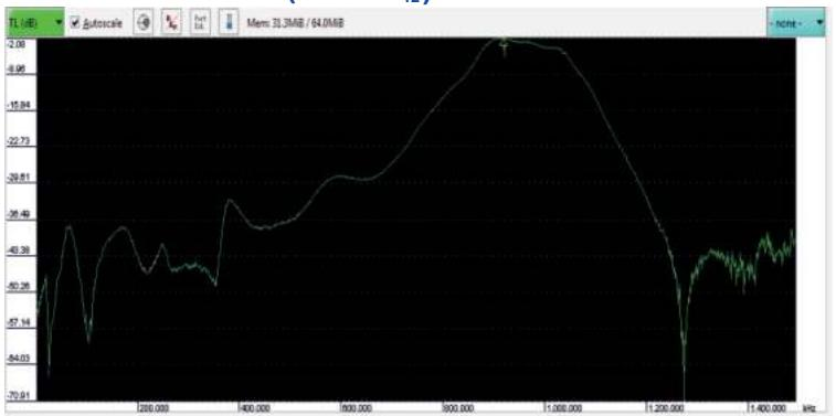
Graph shows transmission coefficients of Hair pin band pass filter and its insertion loss S<sub>21</sub> value is 2dB at 900 MHz
