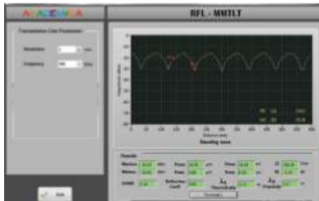
Standing wave @900MHz under OPEN Condition
