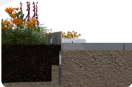
Standard method to compacted MOT Type 1 sub-base or similar material
