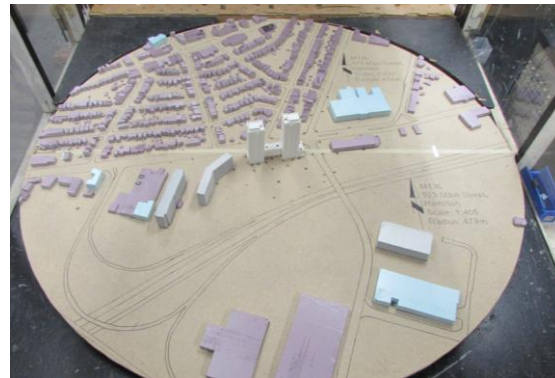
Image 3A: Wind Tunnel Model of the Site and Existing Surrounding Buildings – November 2024
