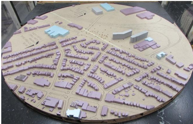
Image 3A: Wind Tunnel Model of the Site and Existing Surrounding Buildings – November 2024
