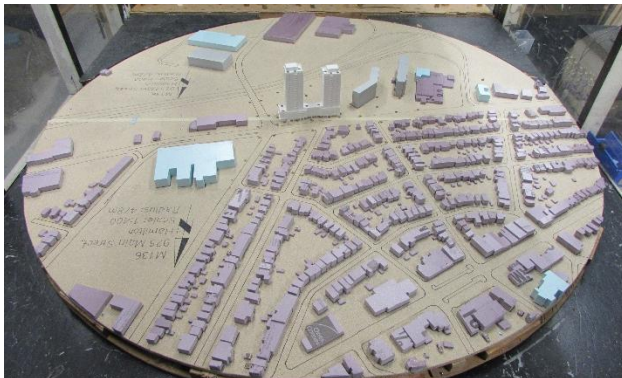
Image 3A: Wind Tunnel Model of the Site and Existing Surrounding Buildings – November 2024
