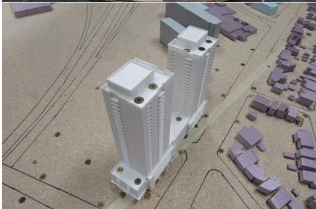
Image 3B: Wind Tunnel Model of the Proposed + Existing Surrounding Buildings – April 2026
