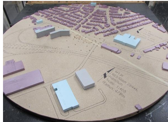
Image 3A: Wind Tunnel Model of the Site and Existing Surrounding Buildings – November 2024
