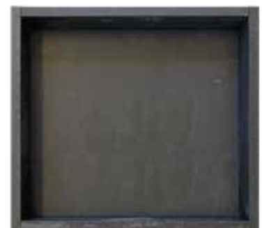
Plastic sample form: 320 x 300 x 40 mm
