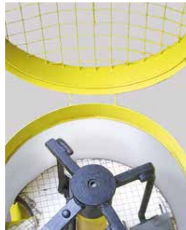
Wear protected tank of the Kalenborn forced circulation mixer
