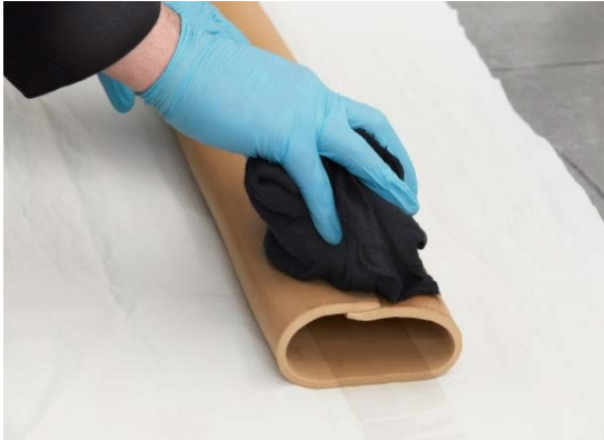
5, Applying solvent on the tube
