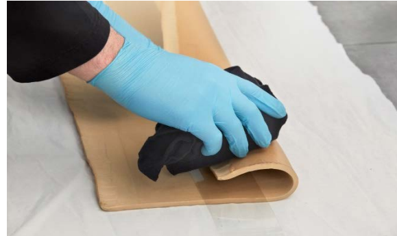
2, Applying cement (or solvent)
