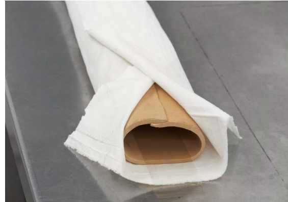
6, Wrapping the tube with Cloth Liner
