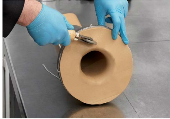
14, Placing Flange cover to Flange face
