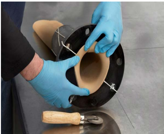
11, Flaring Tube over face of flange
