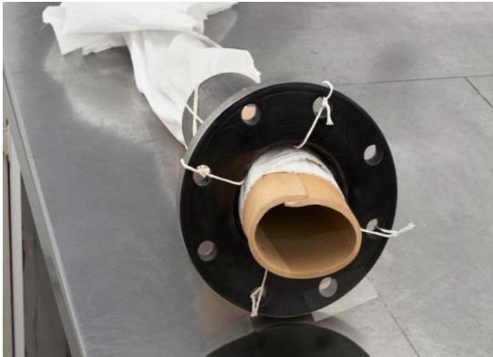
9, Removing the Cloth Liner
