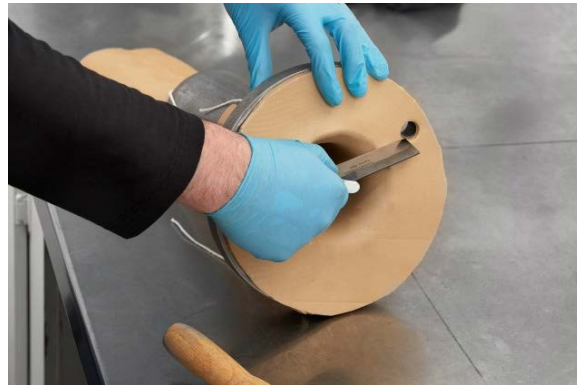
16, Cutting rubber out of bolt holes
