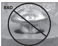
OVAL NECK OF BOLT NOT SEATED PROPERLY
