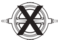
Incorrect Orientation for Horizontal Installation
