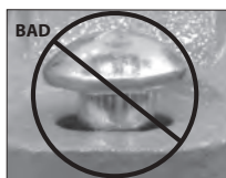
OVAL NECK OF BOLT NOT SEATED PROPERLY
