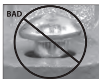
OVAL NECK OF BOLT NOT SEATED PROPERLY
