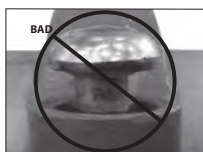
OVAL NECK OF BOLT NOT SEATED PROPERLY
