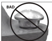
OVAL NECK OF BOLT NOT SEATED PROPERLY
