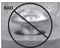
OVAL NECK OF BOLT NOT SEATED PROPERLY
