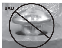
OVAL NECK OF BOLT NOT SEATED PROPERLY
