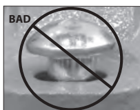
OVAL NECK OF BOLT NOT SEATED PROPERLY
