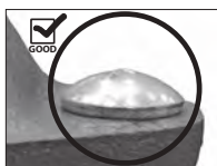
OVAL NECK OF BOLT SEATED PROPERLY
