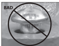
OVAL NECK OF BOLT NOT SEATED PROPERLY
