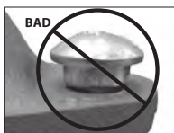
OVAL NECK OF BOLT NOT SEATED PROPERLY
