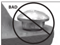
OVAL NECK OF BOLT NOT SEATED PROPERLY
