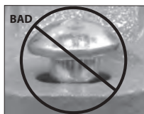
OVAL NECK OF BOLT NOT SEATED PROPERLY
