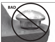
OVAL NECK OF BOLT NOT SEATED PROPERLY
