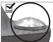
OVAL NECK OF BOLT SEATED PROPERLY
