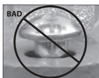
OVAL NECK OF BOLT NOT SEATED PROPERLY
