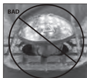
OVAL NECK OF BOLT NOT SEATED PROPERLY
