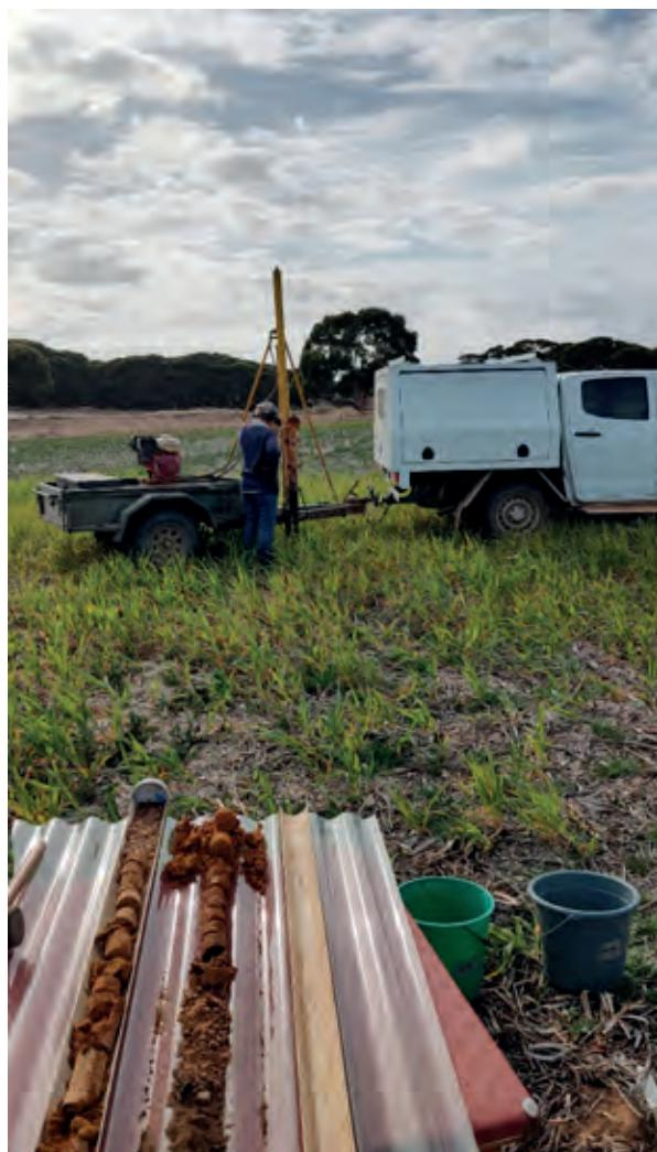
Figure 4: Soil coring & sampling at
