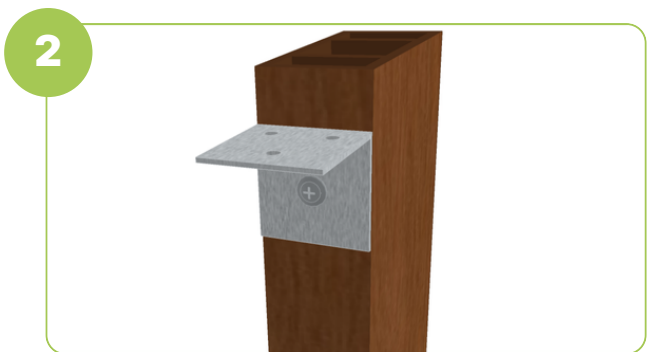
Secure metal angle plates to the drilled holes using wood screws at designated points.
