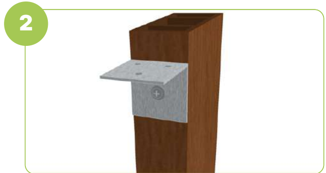
Secure metal angle plates to the drilled holes using wood screws at designated points.
