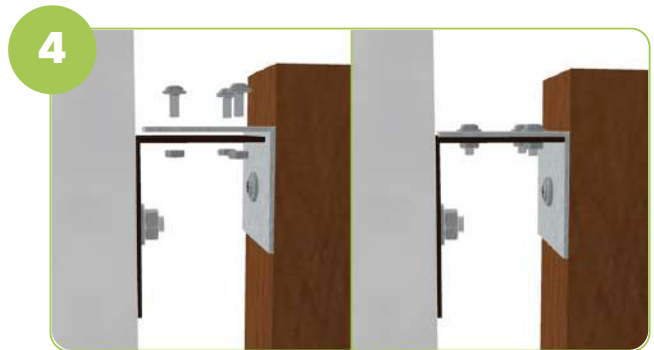
Attach the WPC outdoor columns to the metal clips using the metal angle plates and fasten them with core bolts and nuts.
