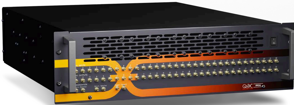
Figure 2 Rendering of FFCU rack mount unit with 32 RF I/Os
