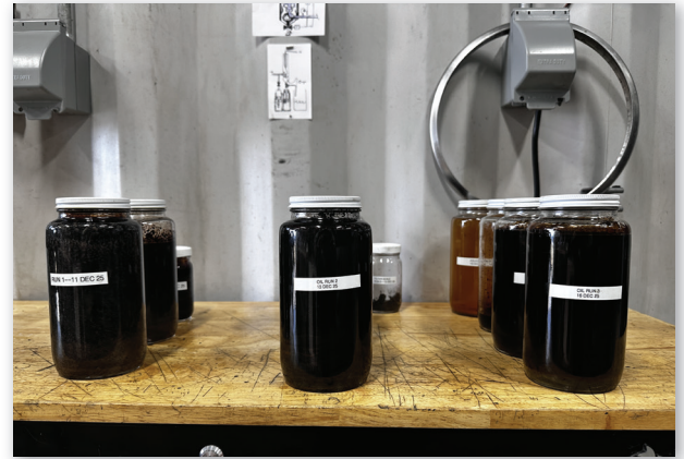
HTL process outputs: biocrude oil, aqueous effluent and blowdown solids.
