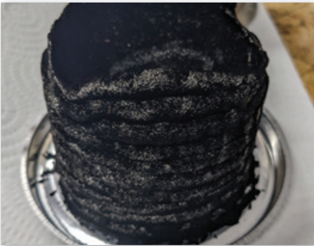
Exhaust soot collected for PFAS analysis following internal combustion and power generation with blended HTL biocrude and biodiesel.
