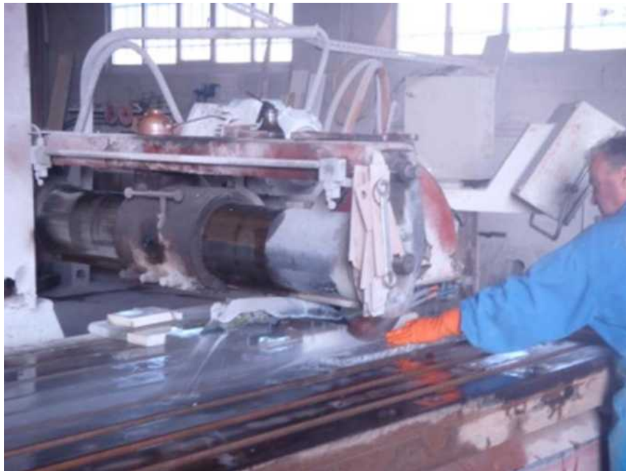
Figure 10.4 Core Being Cut in a Dimension Stone Facility
