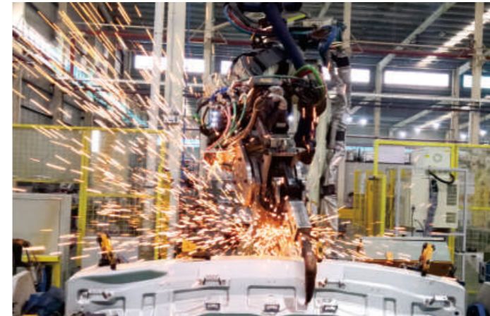
Center console bracket spot welding
