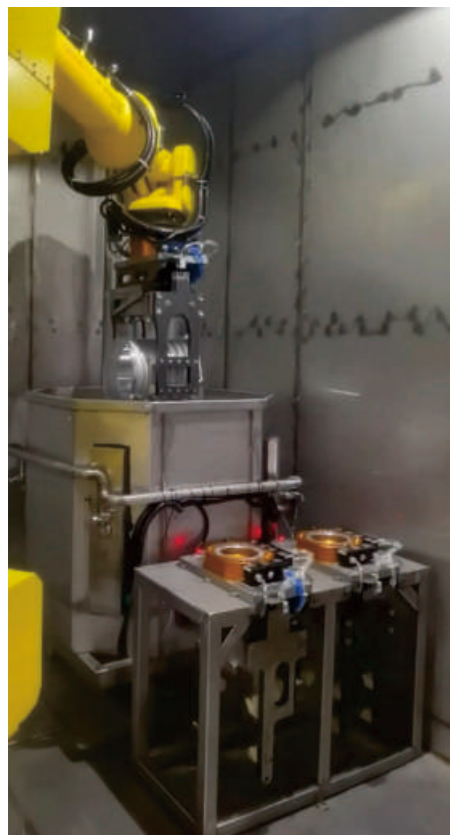
Motor housing cleaning
