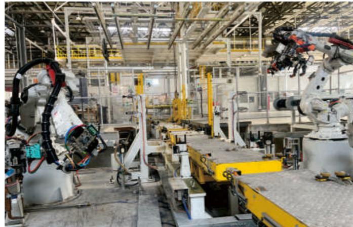
Body welding main line
