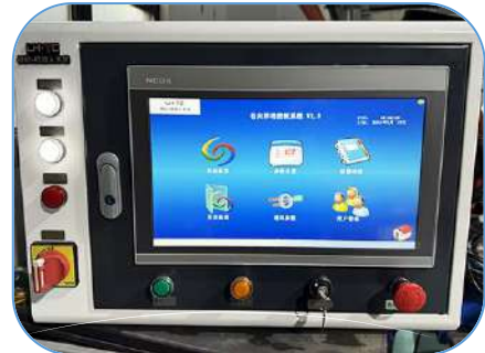
Force control floating grinding control system
