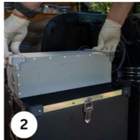
2 Lift heating loop off the top of the solids bin in the aging position.
