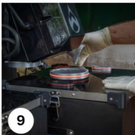
9 Remove vent and slide full bin into aging position.
