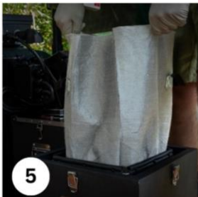
5 Withdraw the bag of aged solids and dispose of them.
