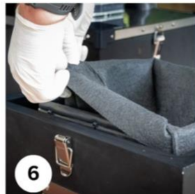
6 Insert new solids bag and fold top of the bag over the basket lip.
