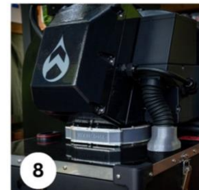
8 Unlatch collar from the neck of the full bin.
