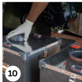
10 Remove bin cap from the now empty bin and place it on the full bin.
