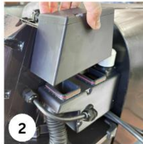
Rock carbon filter forwards and backwards to loosen and remove.
