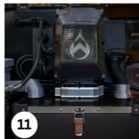
11 Move empty bin into the filling position and reattach collar, vents, and heating loop.
