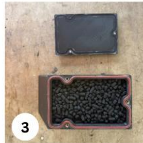
Empty used carbon and refill with fresh 4mm pellet activated carbon media.
