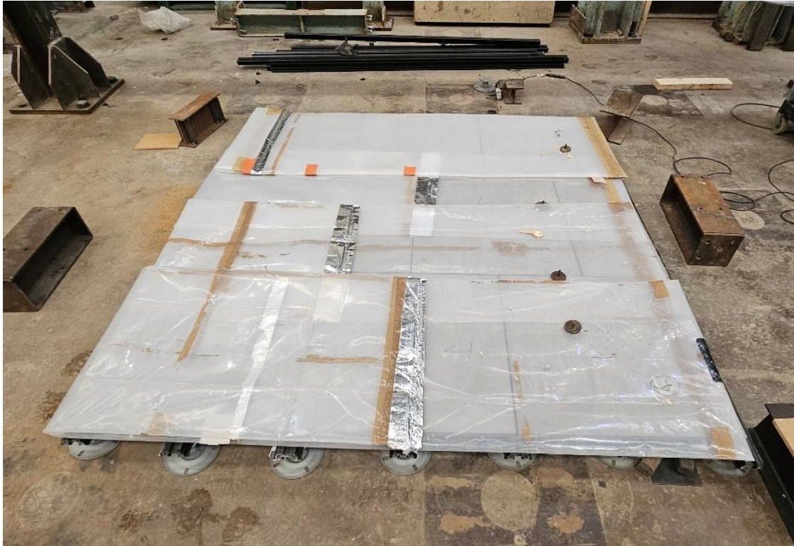
Plate 7 – Sample with Airbags Installed
