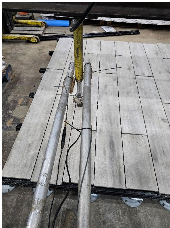
Plate 2 – Point Load Test Set-Up Farrino Tiles
