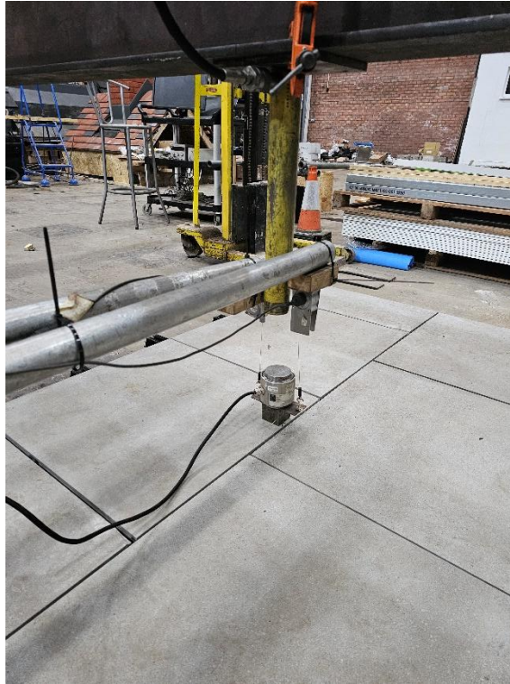
Plate 1 – Point Load Test Set-Up Atria Tiles
