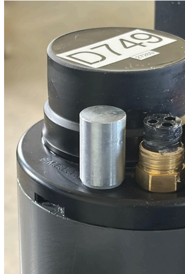
Left: Zinc anode bonded to tanks & valve. Right: Endcap Zinc anode, which protects bulkhead connector & vent.
