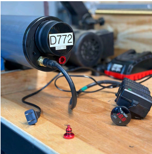
Checking Battery voltage using battery charger - NOTE: Battery charger is UNPLUGGED & vent plug has been REMOVED
