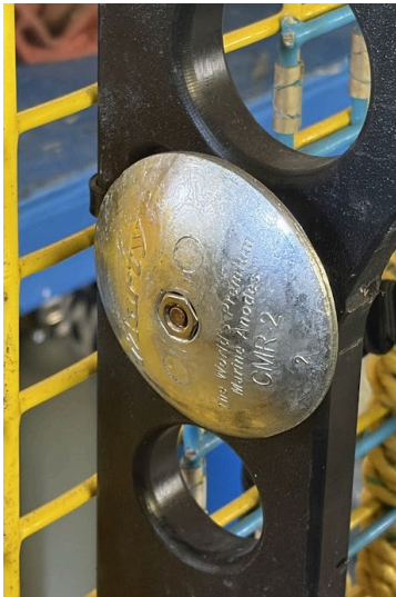
Left: Zinc anode bonded to tanks & valve. Right: Endcap Zinc anode, which protects bulkhead connector & vent.
