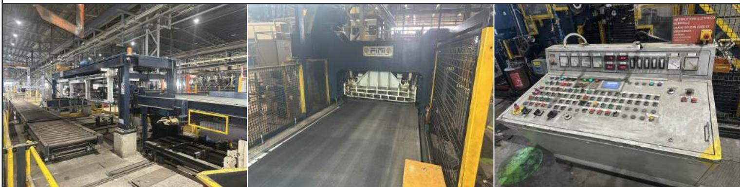
The cut-to-length line provides accurate and efficient processing of stainless steel coils in light to medium thicknesses. Its configuration supports a broad range of cutting lengths, making it a versatile choice for stainless steel sheet production.
