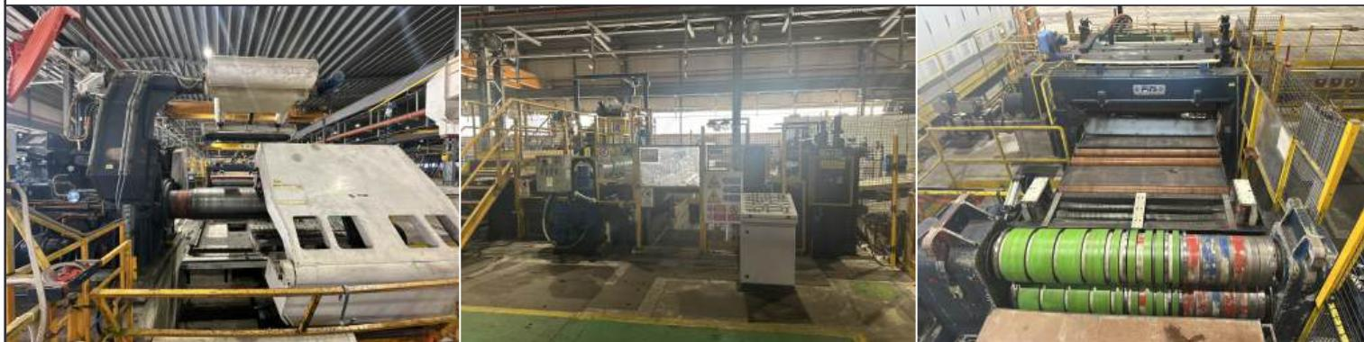
Heavy-duty stainless steel slitting line for coils up to 25 t, designed for reliable processing in the 0.5–5 mm thickness range. Completely revamped in 2022 with CE certification, it combines robust mechanics with upgraded controls, making it suitable for demanding stainless steel service centre and mill applications.
