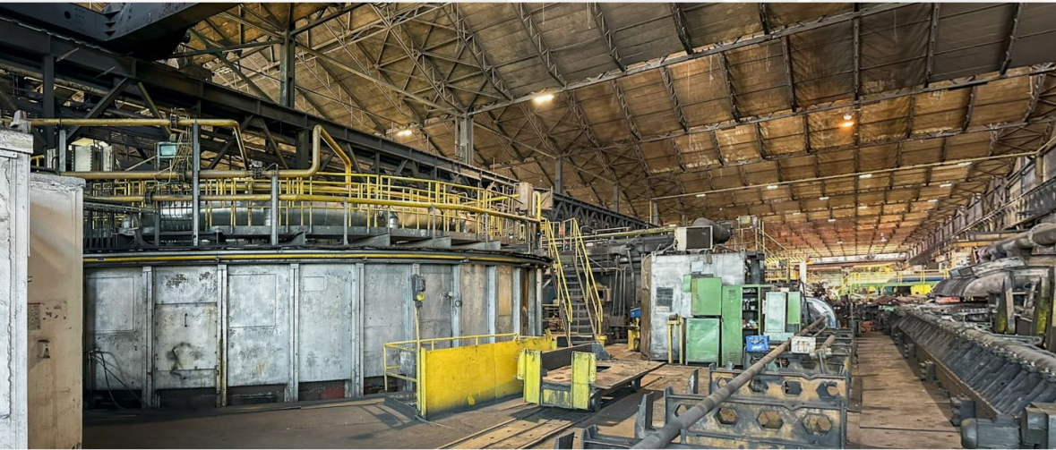
Manufacturer: Bowim Model: - | YoM: 1965 | Overhaul: 2006 Utilities: Natural gas, Water, and Compressed air Drive: Electric Drive - 2x 15 kW Motors, 1400 RPM Effective Shell Area: 104 m² Rotary Shell Dimensions: 15800/2700 mm Charging Temperature: 1250°C Fuel Consumption: 1000 m³/h
