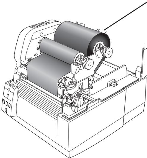
Remove waste ribbon to reveal print head (the head requires cleaning every time the ribbon is replaced).
