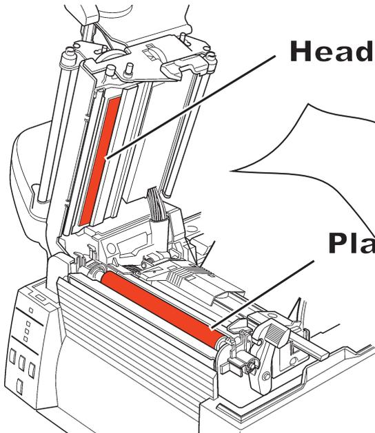
Clean the print head using alcohol wipes by firmly but carefully wiping the head. Also rotate and wipe the platen roller.
