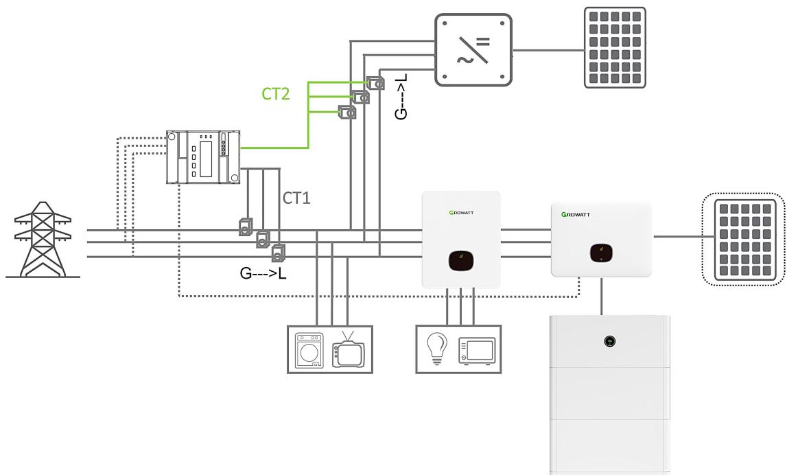
In the above scheme, Growatt inverter can be used to retrofit any brand of third-party system, however, the whole system doesn't have the export limitation function due to the inability to control the third-party inverter.
