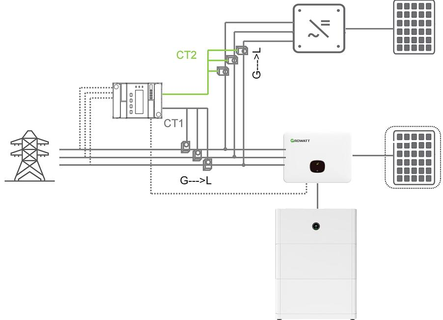
In addition, by installing a SYN Box( SYN 50-XH-30 for MOD-XH(BP), SYN 100-XH-30 for MID-XH), the system is able to switch from on-grid to off-grid, and by connecting critical loads to the SYN box to ensure continuous power supply to the critical loads in case of power outage.
