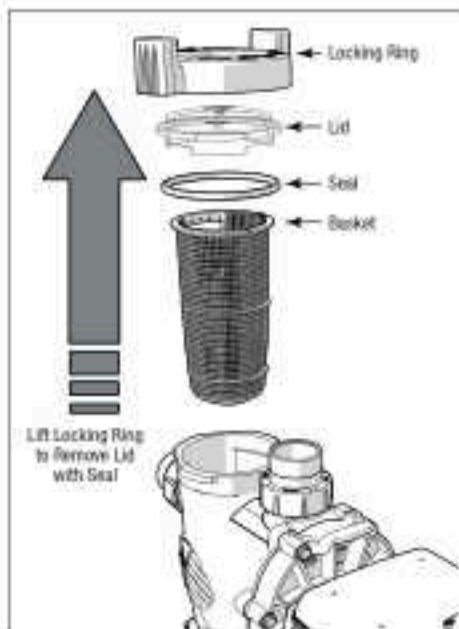
Figure 18. Remove Pump Lid
