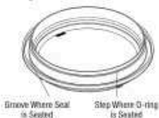
Figure 16. Placement of Blue Pressure Test O-ring
