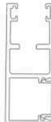
Profile of EA ® 44mm (1.73") End Retention Side Rail
