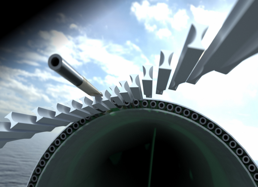
Gurit's pultruded root reinforcements offer market-leading secondary bonding properties and superior fracture toughness. – Photo Gurit
